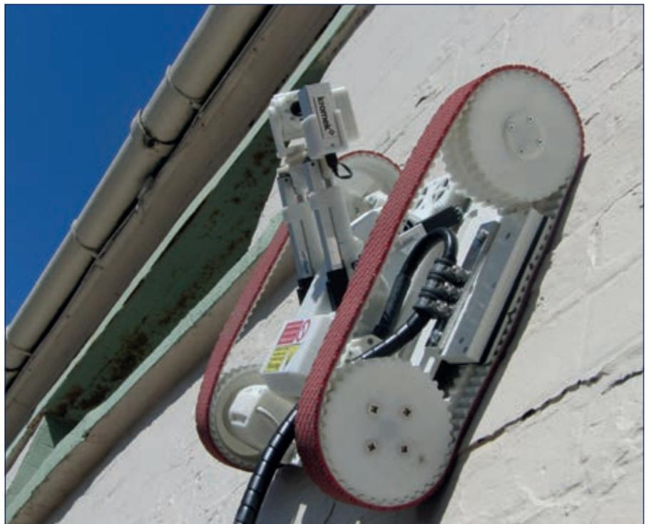
**The WallRover B is capable of climbing walls, but falls short of Robug III's aspiration to lug a 100kg payload behind it. (Photo: WallRover)**
