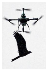
Calcutta police tested their eye in the sky on Tuesday for aerial surveillance during Durga Puja. The unmanned aerial vehicle can be controlled from a mobile base station. It can hover at 250m and capture images within a 5km range. The drone has a night vision camera too. "If the UAV works fine, it will be used even after Durga Puja. We paid over Rs 38 lakh for this DRDO-made device. We will get more, if needed," said city police commissioner Surajit Kar Purkayastha. Picture by Sanjoy Ghosh
