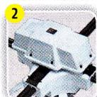
**2** The battery, fitted on top, allows it to fly for upto half an hour. Just below the battery is the brain of the product. It is a small and extremely light auto-pilot
