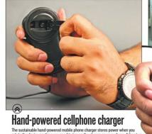
The sustainable hand-powered mobile phone charger stores power when you rotate the device anytime you need to top up the charge on your phone. It has two modes: crank (wind-up) or not (101-on). One minute of rotating the handle gives about three minutes of talktime and about 30 minutes of stand-by time.
