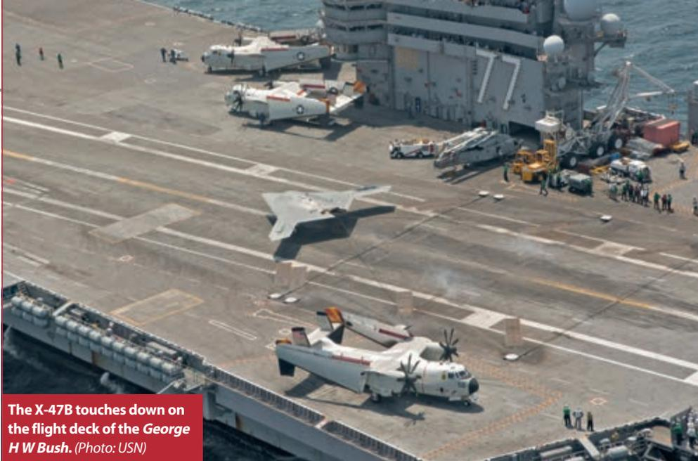
The X-47B touches down on the flight deck of the *George H W Bush*. (Photo: USN)
